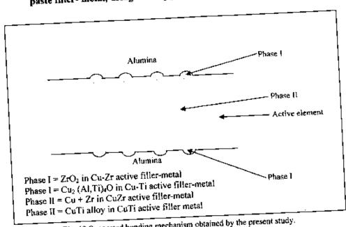
Fig. 13 Suggested bonding mechanism obtained by the present study.
